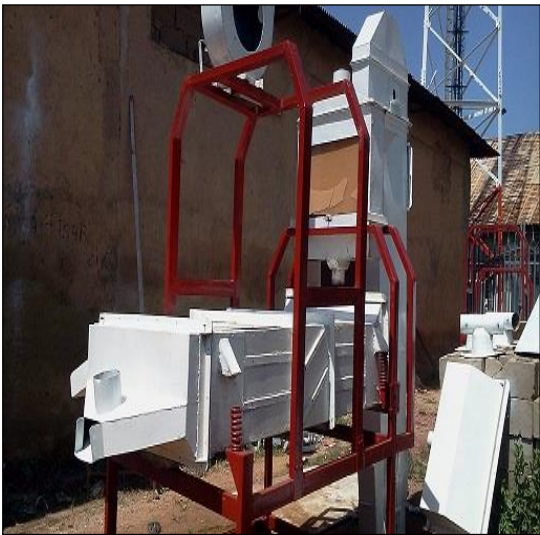
Components of the integrated sesame seed cleaning machine
