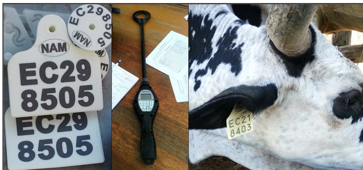
Figure 21: Nam-LITS ear tags, from left to right: visual and circular (RFID) tag, RFID reader and visual tag in ear.
